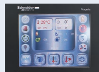
Touch screen control panel with PLC. Panel de control con pantalla digital PLC.
